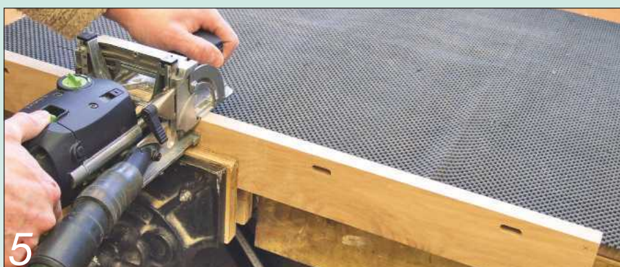
5 I cut the mortises in the face-frame stiles using my Festool Domino joiner
