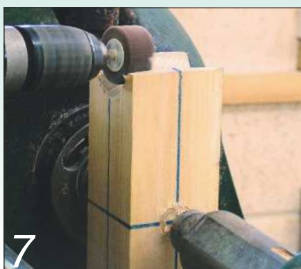
7 Stop the lathe and sand the cove smooth with a small rotary sanding drum
