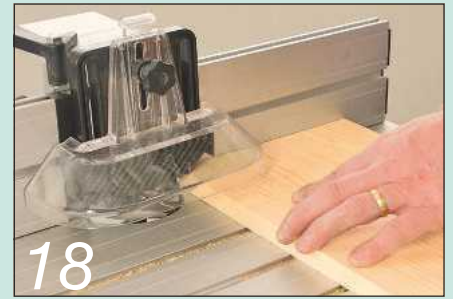
18 Make the end-grain cuts with several passes
