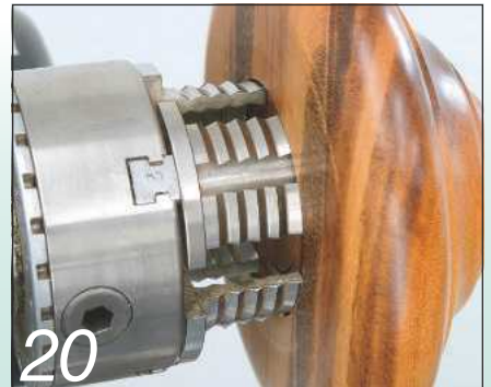
20 'Shark' jaws have a deep gripping surface and improved rear access
