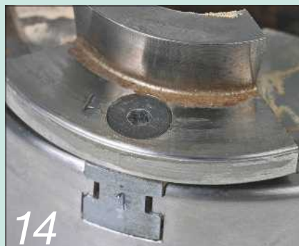
14 You'll find that each jaw and carrier on the chuck is numbered
