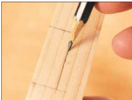
6 Run a sharp pencil along the gauged line to make it more clearly visible
