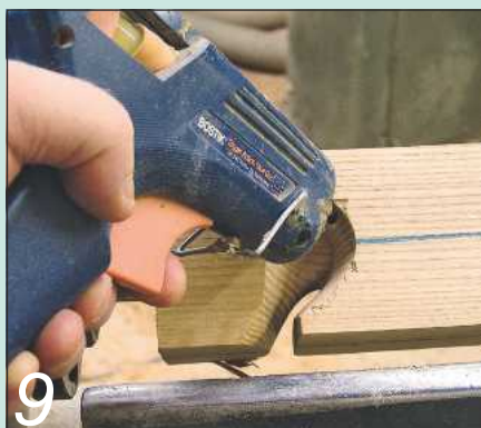
Turn a 22mm spigot on the second blank and glue it into the drilled hole in the vase
