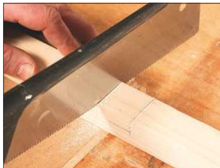
7 Hold the rail on a bench hook and use a tenon saw or pullsaw to cut down to the gauged line at each side of the joint
