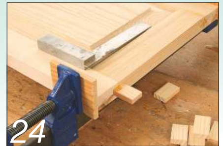
24 ...before gluing each frame round its panel
