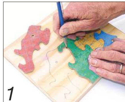
1 Make mdf patterns of the shapes, then draw their outlines directly on the wood
