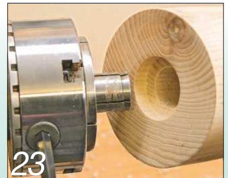
The standard pin chuck is an ideal way of holding pre-bored work
