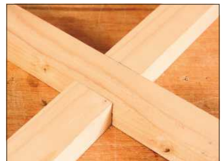
11 Apply glue sparingly to the two notches and assemble the joint. Check that it's square, then set it aside for the glue to dry
