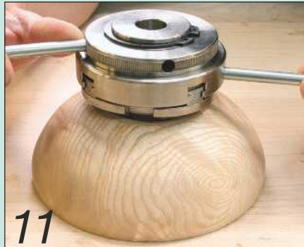
11 The work has to be mounted horizontally while it is off the lathe
