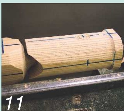
Keep the last 25mm or so at each end of the piece nearly square
