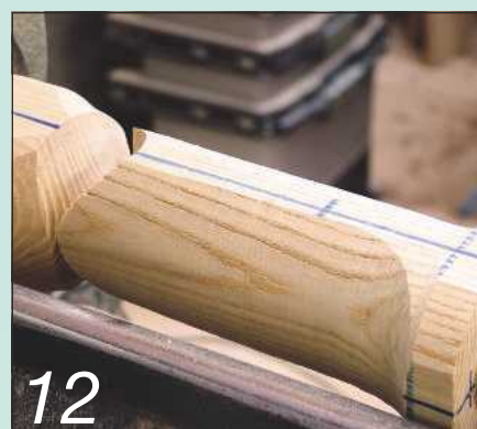
Mount the piece on one pair of off-set centres and turn one side of the vase
