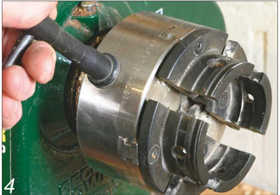
4 Hold the work with one hand and tighten the chuck with the other
