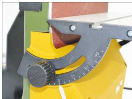
There is a clearly marked scale for setting the angle of the table
