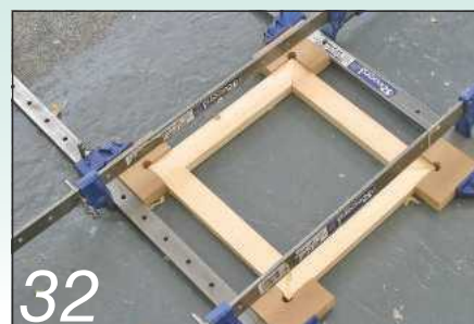
Cut and assemble the overhanging top frame
