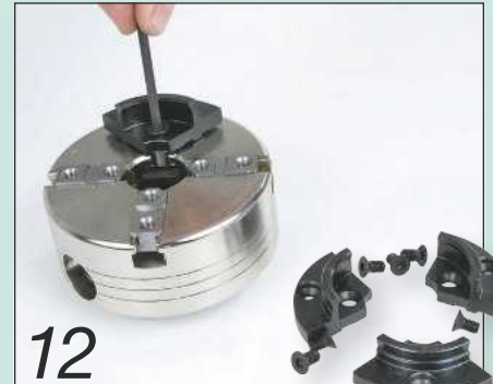
12 The jaws are normally fixed with a couple of small machine screws...
