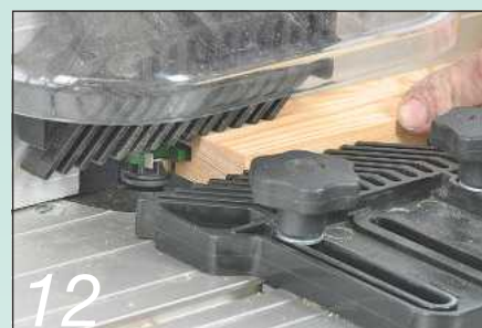
12 Use featherboards to guide the workpieces...
