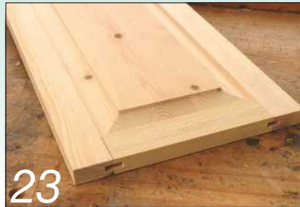
23 Assemble the panels dry to check the fit...
