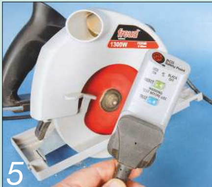
5 If your workshop isn't RCD-protected, always plug your saw into an RCD adapter like this
