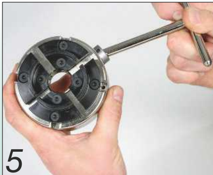
5 Some chuck keys have a swivel action that's easier to use
