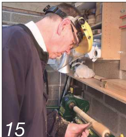
15 A safety visor is the minimum of protective equipment a turner should wear
