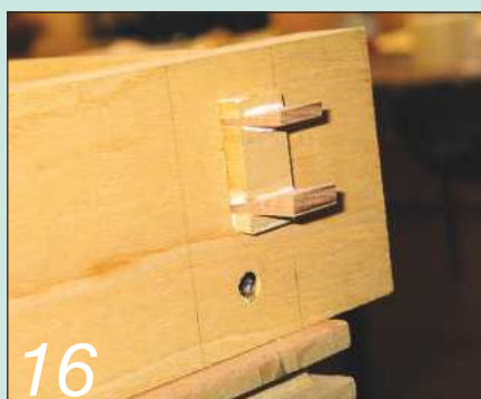
The outer frames have wedged tenons at the top corners for extra strength
