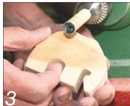
3 Sand all the cut edges smooth. A small-diameter sanding drum is very useful for this
