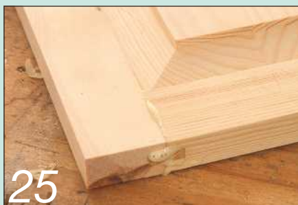
Cut small tongues to fill in the grooves
