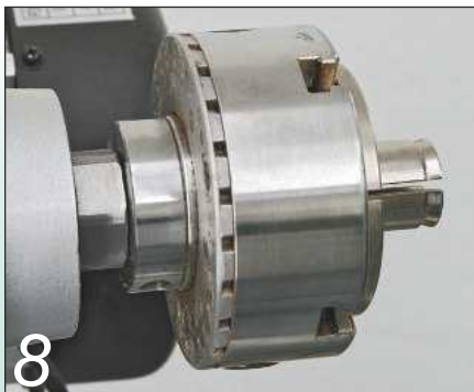
8 The boss will often extend the amount of overhang on the chuck
