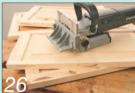
Each corner joint is made with three biscuits
