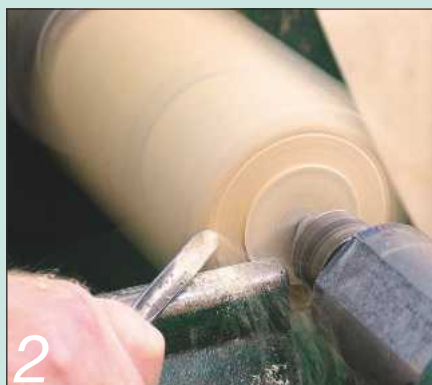
2 Use a \frac{3}{8} in spindle gouge to turn a spigot on the tailstock end of the blank
