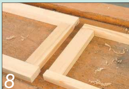
8 Lay out the components to check overall sizes
