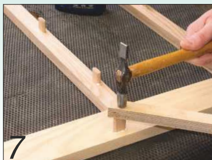
7 Tap the loose tenons into the face-frame mortises before fitting the frame
