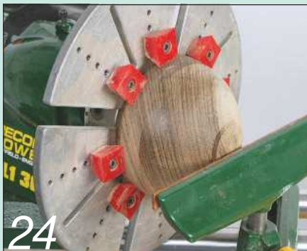
24 Large jaw plates are worth buying if you do a lot of bowl work
