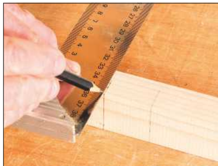
4 Turn the rail on its side and use the try square again to extend both of the marked lines approximately halfway across the edge
