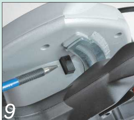
9 Blade changing has been made much easier with the introduction of the spindle lock
