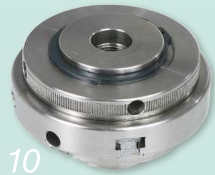
10 The result is a slimline chuck with very little overhang
