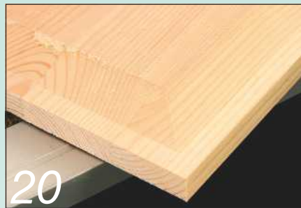
20 ...removed by the second cut along the grain
