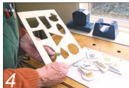
Separate the boards, remove the pattern and sand all the cut edges smooth
