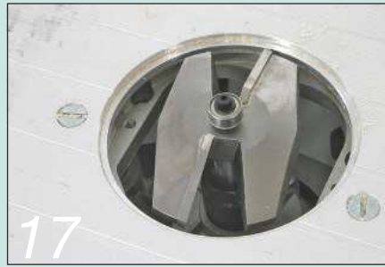
17 Check the clearance in the table aperture
