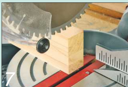
7 Cut matching components to length in batches
