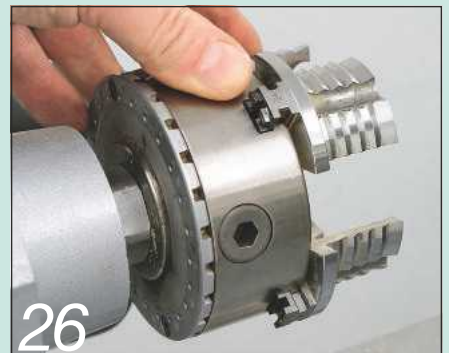
26 The best scroll chucks have a jaw restraint as a safety feature
