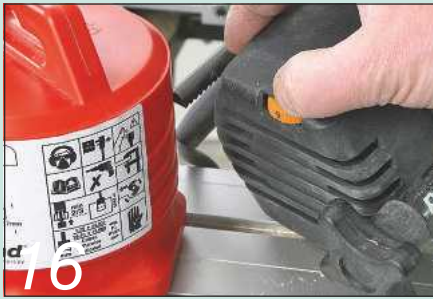
16 Set the router speed to suit the cutter
