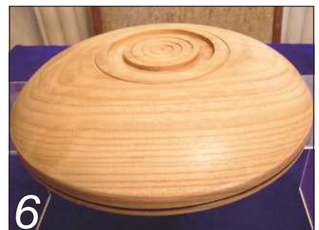
The chucking spigot looks good on the finished article with a few decorative rings added
