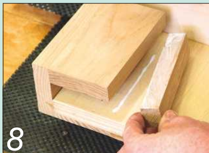
8 Reinforce the stile return with an offcut of ash so it looks like a solid post
