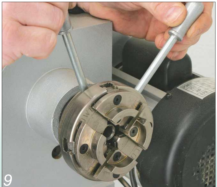
9 Instead of a single chuck key, this type uses a pair of levers
