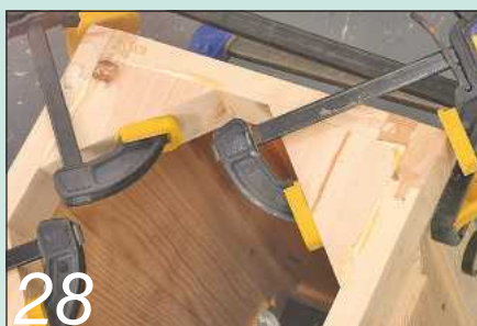
Fit corner braces to support the planter base
