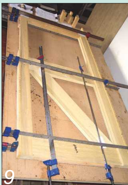
9 Each door frame can now be glued up, cramped and set aside to dry
