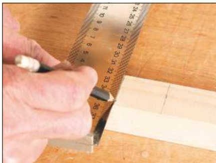
3 Remove the divider carefully so you don't disturb the try square and mark the second line against it to define the joint width
