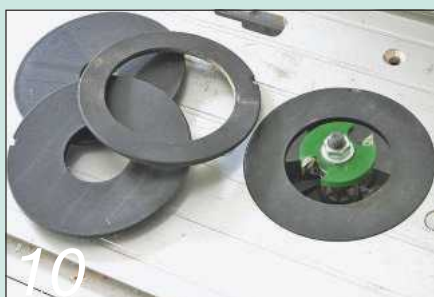
10 Select a table insert that will clear the cutter
