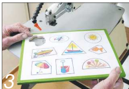
Thread in the blade, clamp it and cut out one shape. Repeat this for the other pieces
