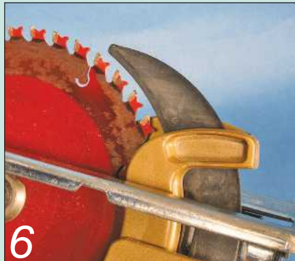
6 The riving knife prevents the blade from jamming in the saw cut. Never be tempted to remove it
