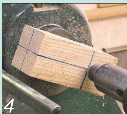
4 Mount the blank transversely between the centres on the two sides
