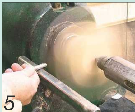
5 Use a spindle gouge to cut a cove in the end of the rotating blank
