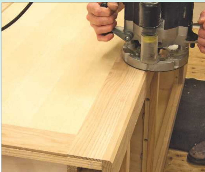
12 Chamfer and groove the lengths of cornice moulding using a router table
