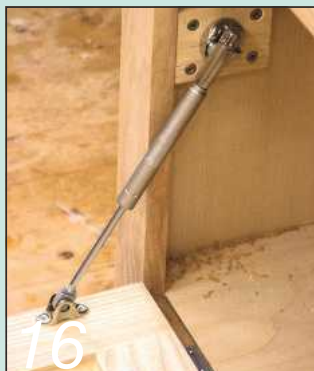
The lower door is fitted with a drop lid stay, mounted on a spacer block
