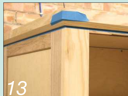
13 Hold the cornice mouldings in place with low-tack tape until the glue sets
