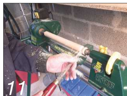
11 The blind spigot on the end of the towel roller is cut in with a parting tool
