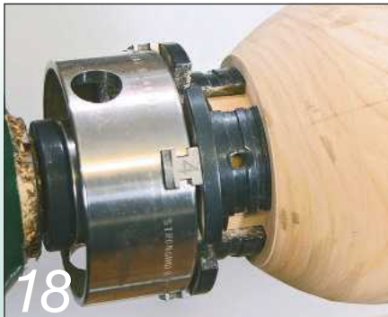
18 It can also grip a spigot on the end of a larger-diameter piece
