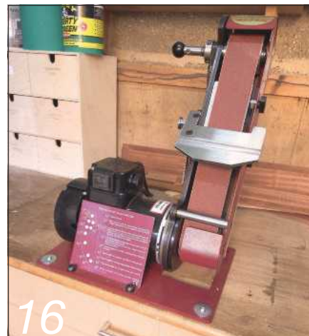
16 I'm hoping my Sorby ProEdge machine will help me explore sharpening safely in the future
