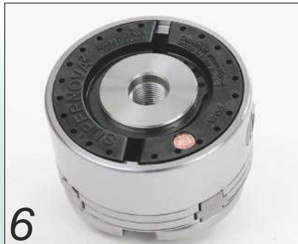
6 Some chucks have the back bored to a specific thread...
