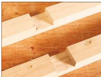
10 Check the fit of the completed components, and pare away more waste as necessary to get a perfect fit
