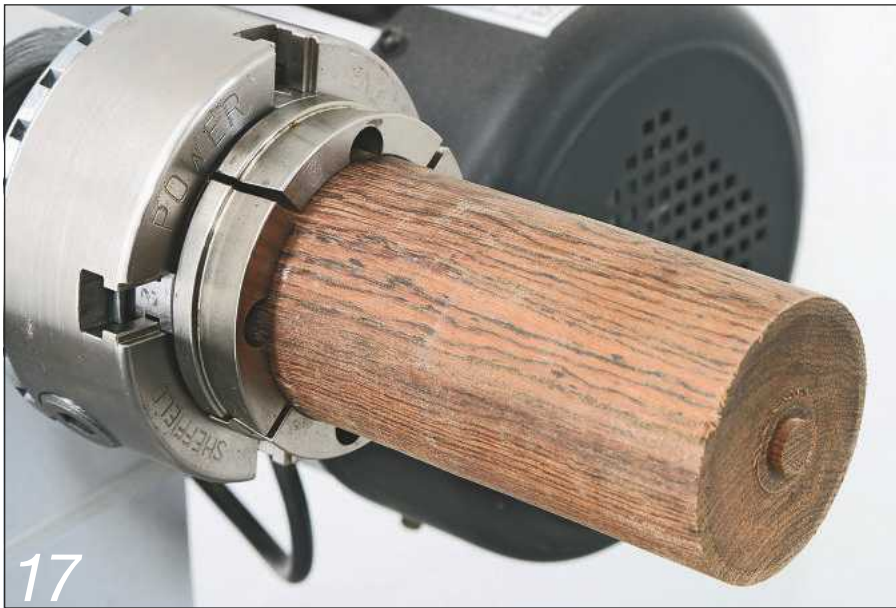
The chuck can grip round stock such as a complete cylinder
