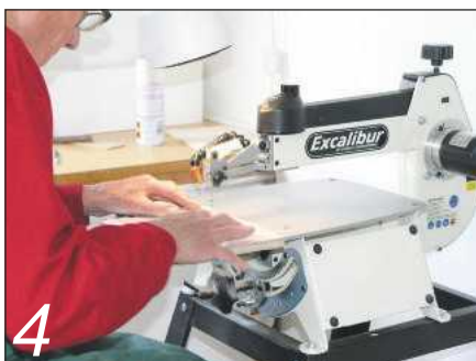
Tape the vertical strips back together and cut the five horizontal ones in the same way
