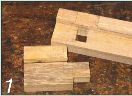
1 Before cutting anything for real, I made a test joint for the outer door frames
