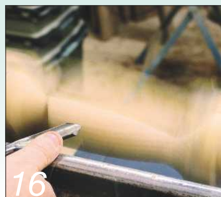
I found it best to taper the blank towards the base with a spindle gouge
