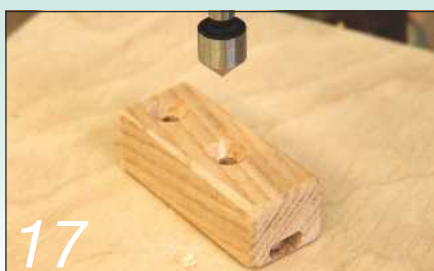
Prepare stop blocks containing a rare-earth magnet and countersink them
