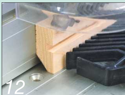
12 Chamfer and groove the lengths of cornice moulding using a router table
