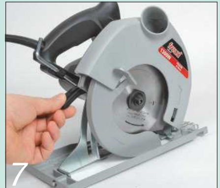
7 Set the depth of cut so that only three teeth at a time cut through the material
