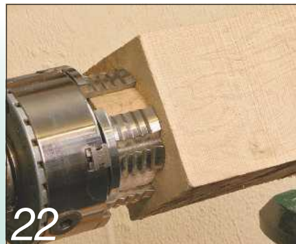
The 'shark' jaws' grip on the work is amazingly firm and rigid
