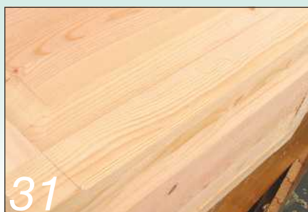
Chamfer the corners in line with the rails
