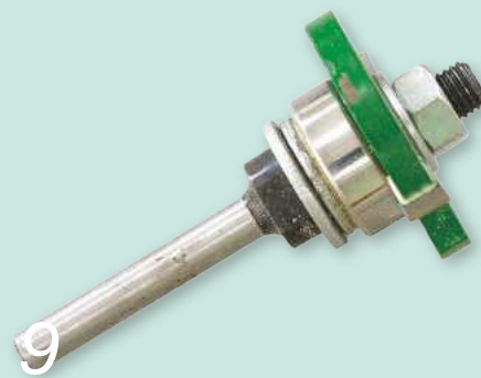
9 Use a grooving cutter mounted on an arbor
