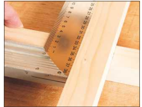
2 Lay the divider on the rail with its edge on the marked line and butt the try square up against it
