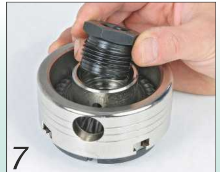
7 ...while others are supplied with a range of separate inserts
