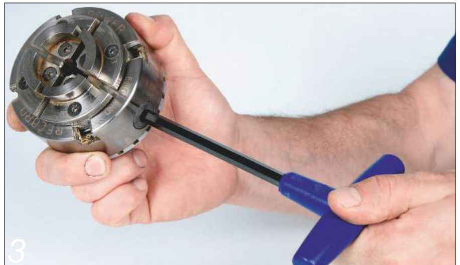
3 The scroll is operated by a hex wrench or a conventional chuck key
