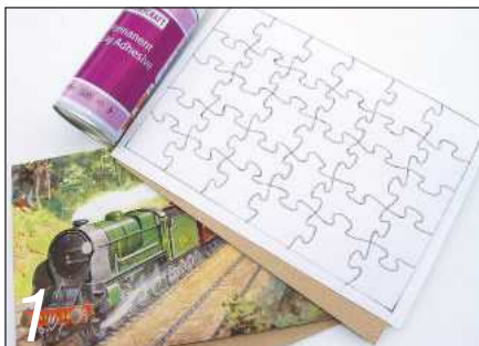
Use aerosol adhesive to stick the image to the plywood and the pattern to the mdf
