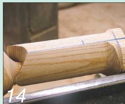
Continue turning until you reach the centre line along the vase's length
