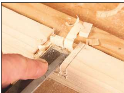
9 Pare away the waste wood with a chisel. Then mark out and cut the notch on the dividing component in exactly the same way
