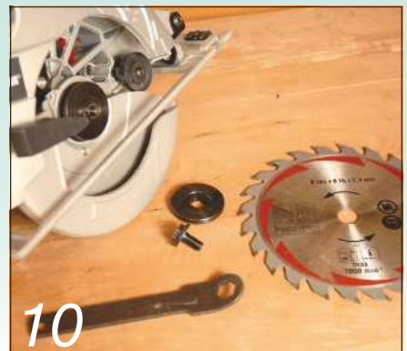
10 Remove the arbor bolt and washer and retract the blade guard to release the blade
