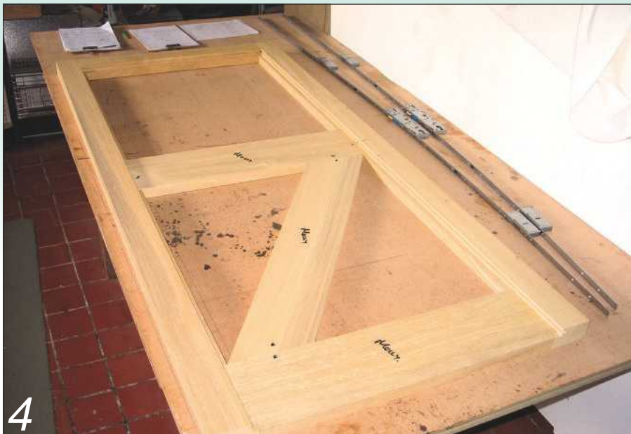
4 Each door has a single brace, fitted between the middle and bottom rails
