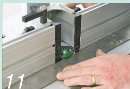
11 Bring the router fences in close to the cutter
