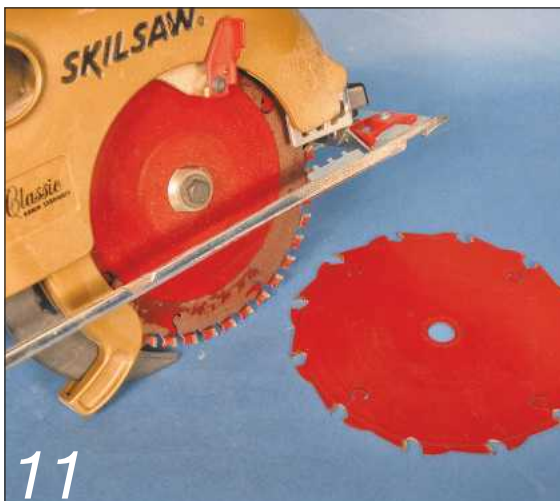
11 A fine cross-cut blade fitted to the saw, and a rip blade in the foreground
