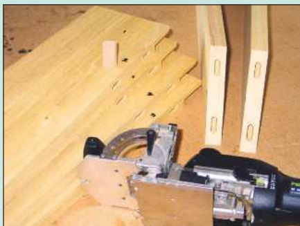
1 Before cutting anything for real, I made a test joint for the outer door frames
