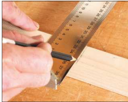
1 Use a try square to mark the position of one edge of the dividing component on the rail
