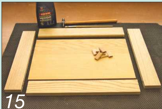
Prepare the door stiles, the rails and the centre panel ready for assembly
