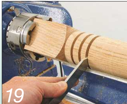
19 The chuck can also be used for holding square-section work
