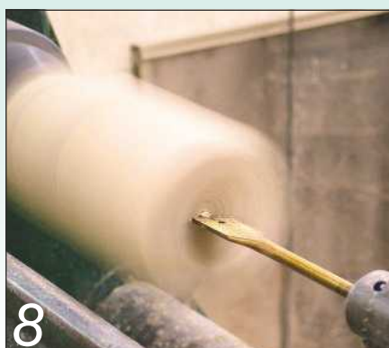
8 Drill a 22mm diameter hole about 50mm deep in the centre of the cove
