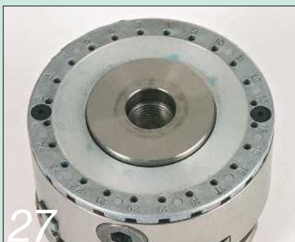
On some scroll chucks the backplate incorporates a dividing head
